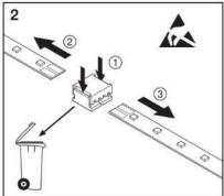
In order to maintain adequate electrical contact, the connectors are designed for single use. However, to reuse the connected PCB, a removal is possible but will result in the destruction of the connector.
