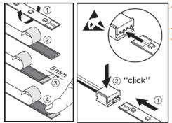
For electrical connection of the LINEARlight FLEX, both, module and connector must be positioned with the correct side up as shown in the graphic
