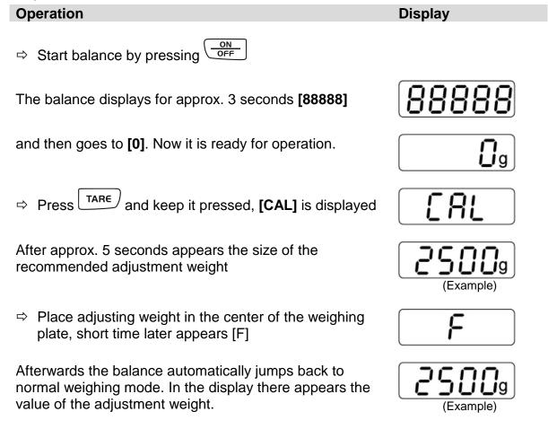
An error during adjustment or the use of an incorrect adjusting weight will result in an error message "**CAL E**". Repeat adjustment.
