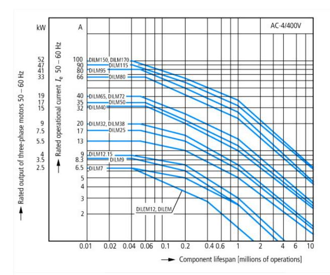
Extreme switching duty Squirrel-cage motor Operating characteristics Inching, plugging, reversing Electrical characteristics Make: up to 6 x rated motor current Break: up to 6 x rated motor current Utilization category 100 % AC-4 Typical applications Printing presses Wire-drawing machines Centrifuges
