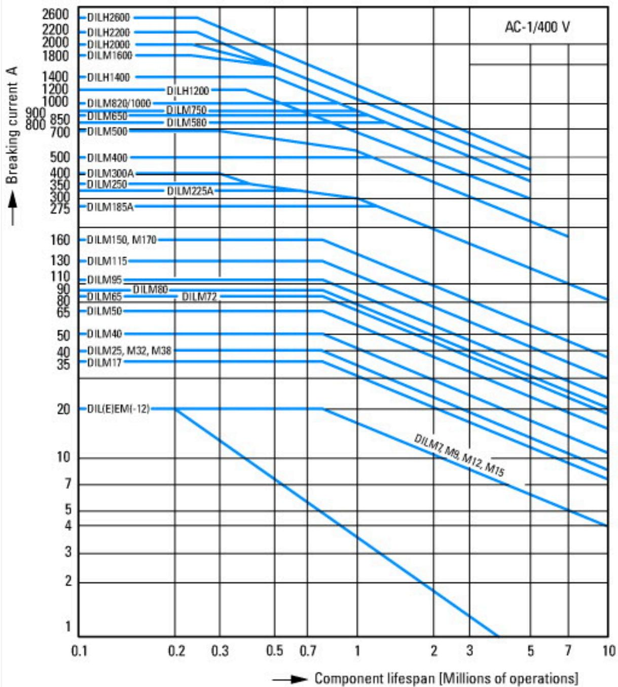
Switching conditions for 3 pole, non-motor loads
