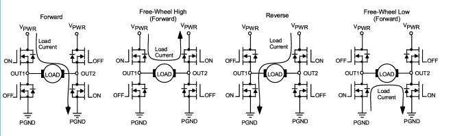
Figure 9. Output operating configurations
