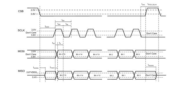
Figure 8. SPI dynamic diagram
