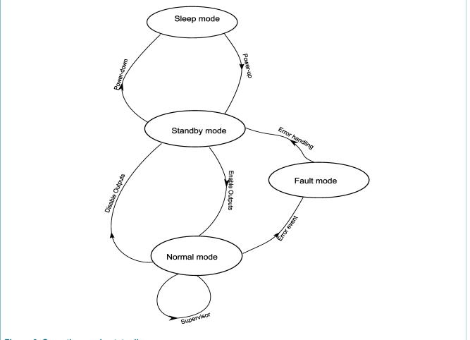
Figure 6. Operating mode state diagram
