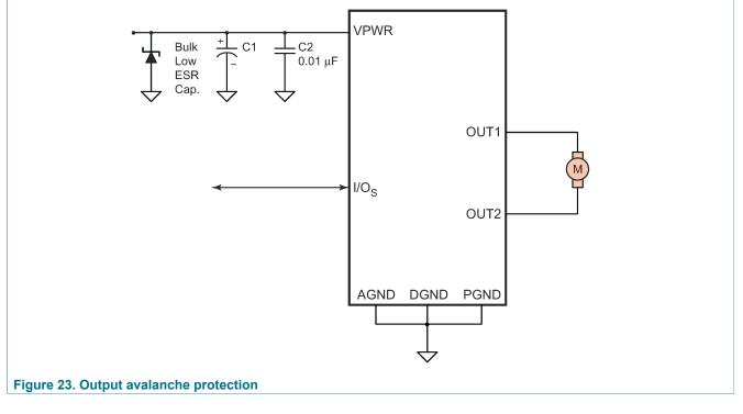
ESR as shown in <u>Figure 23</u>. If ENBL is at logic [1] and the part is in H-Bridge mode, this problem is mitigated by internal overvoltage protection.
