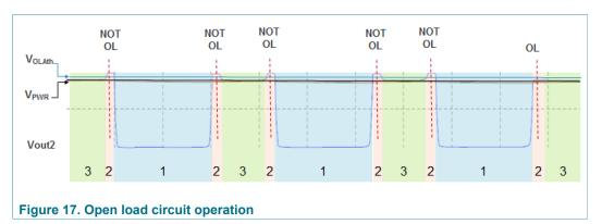
During normal operation, the result of the open load detection window is held until the end of the next detection window. Open load detected in the active mode is a dynamic status which is only cleared by detecting the load is not open or leaving Normal mode.
