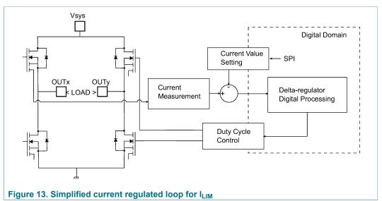
The active current limit threshold is selectable by the SPI in four steps from 5.0 A to 10 A. The active current limit is initiated, and the OC SPI fault status bit is set when the current exceeds the threshold set by the current limit comparator.
