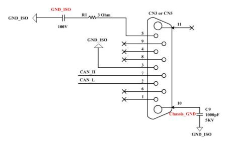
Figure 4.2 PCIE-1680 DB-9 connector schematics
