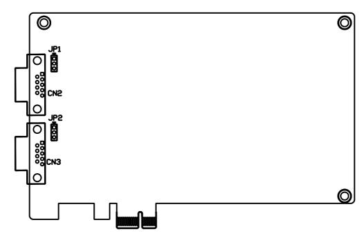
Figure 3.1 PCIE-1680 CAN-bus board silk screen
