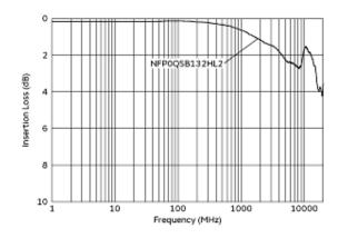
Common Mode Insertion Loss Characteristic (Typical Value)
