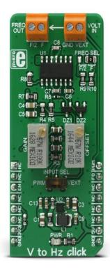
When V to Hz click is operated for the first time, it needs to be calibrated. The click is equipped with two variable resistors for gain and offset fine tuning. There are several steps that should be followed when calibrating:
