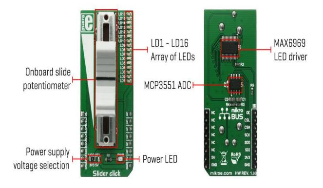
This click board  $^{\text{TM}}$  can work with both 3.3V and 5V, depending on the used MCU capabilities. This can be done by switching the VCC SEL SMD jumper to the desired position.
