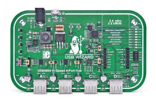
**USB Wizard** is an evaluation and demonstration platform featuring the <u>USB4604</u> USB 2.0 4-Port hub controller. The board has four USB 2.0 downstream ports with individual port power control and overcurrent sense (OCS).
