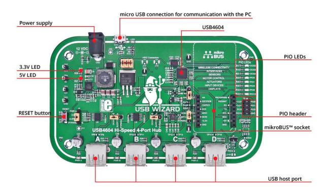
On the bottom part of the board, you'll find 4 USB host ports. With the USB Wizard, you will no longer be running low on USB ports.
