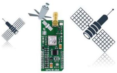
The user wanting to use GPS to determine its position must have an antenna that receives the signals coming from the satellites, and a receiver that translates these signals. The antenna position will be deduced from the measurements of the time delay between the emission time (satellite) and the reception time (receiver) for at least 4 signals coming from different satellites.
