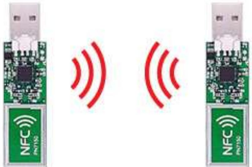
Peer-to-peer mode establishes a two-way communication channel between a pair of NFC-enabled devices. When a user brings two devices close to each other, the two NFC chips establish a P2P connection and exchange data.
