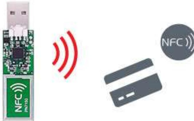
Here, NFC USB Dongle communicates with a passive tag, smart card, or an NFC device operating in card emulation mode. It can both read or write to a tag (although reading is a more common use-case because tags will often be write protected). In this mode, it is USB NFC Dongle that generates the RF field, while a tag or card only modulates it.
