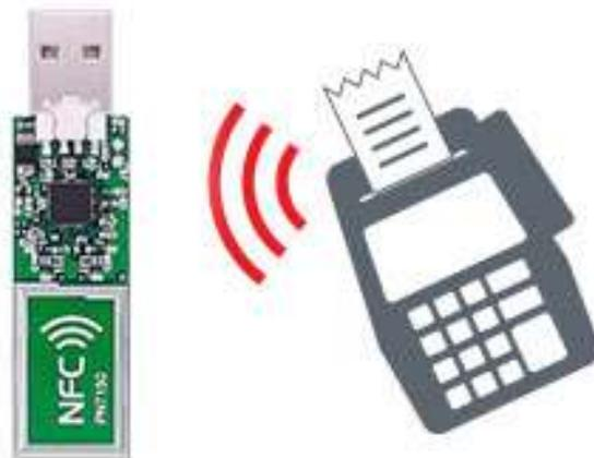
In this mode, NFC USB Dongle emulates an NFC tag. It doesn't initiate the communication, it only responds to an NFC reader. A typical application of the card emulation mode is how people use NFC in their smartphones to replace several cards, badges and tags at once (using the same phone for tollgate check-ins, contactless payments and so on). Card emulation mode, however, is not useful just for smartphones, but for any type of portable device.
