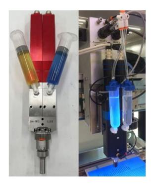
2K coating materials can be applied thinly (50-75µm), however they have been designed, formulated and tested to be applied at much greater thicknesses (250-300µm), to facilitate superior encapsulation of components and component leads.
