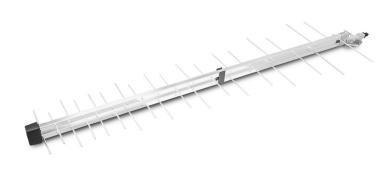
The L36FK Log-periodic aerial has been tuned to reject 5G700 interference above channel 48. Log-periodic antennas are ideal suited for strong to medium signal areas within the primary service area of the transmitter due to their flat response and excellent front to back rejection. The antennas are light weight and specifically designed for low wind loading. The mast-clamp is designed for horizontal or vertical polarisation and suitable for 1" or 2" masts.
