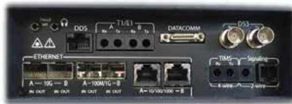
Fully equipped platform. Unused ports can be blanked off.
