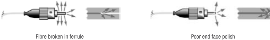
Fibre broken in ferrule
