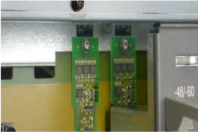
Illustration shows chassis data module 21596-023
