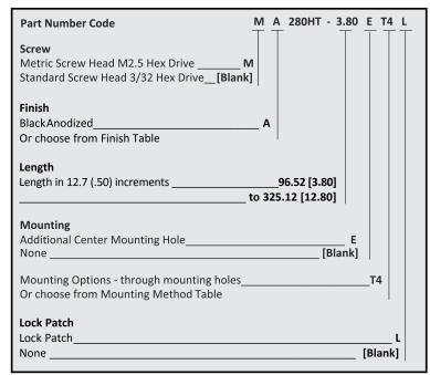
Part Number Code example: A280HT-4.80T4 Series 280HT Card-Lok five piece 121.9 (4.80) long with black anodize finish, 4-40 tapped hole for mounting.
