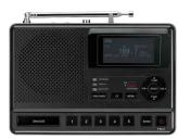
The CL-100 has a graphic LCM (128 \* 64 Pixels Graphic) LCD module with excellent display quality and wide viewing angle. It can scroll LCD display of S.A.M.E. event information. In addition, the CL-100 has dimmer and contrast control adjustment for viewing the display in the dark.
