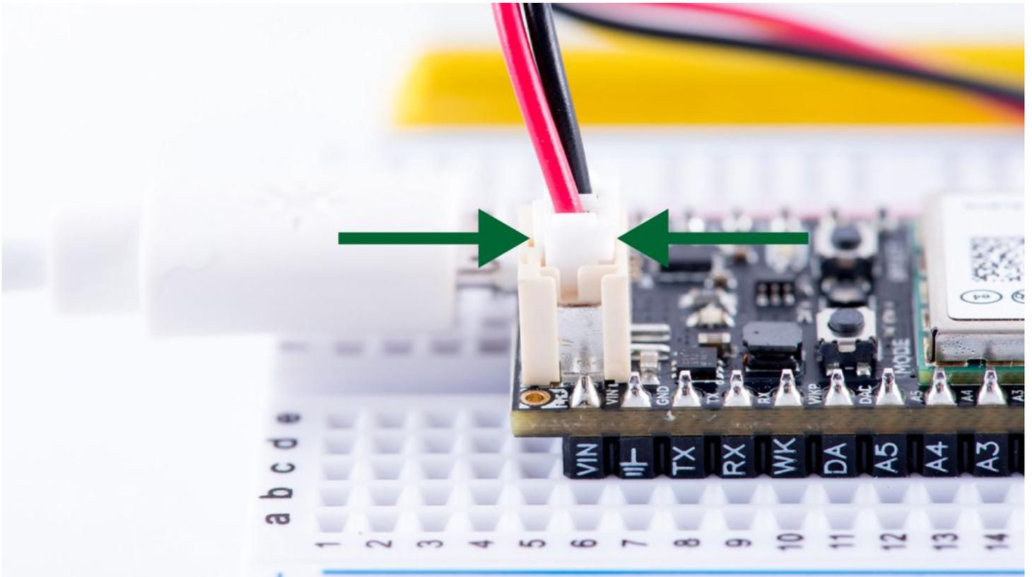
The micro B USB connector on the electron is soldered on the PCB with large surface pads as well as couple of through hole anchor points. Despite this reinforcement, it is very easy to rip out the connector if too much stress is put on in the vertical direction.
