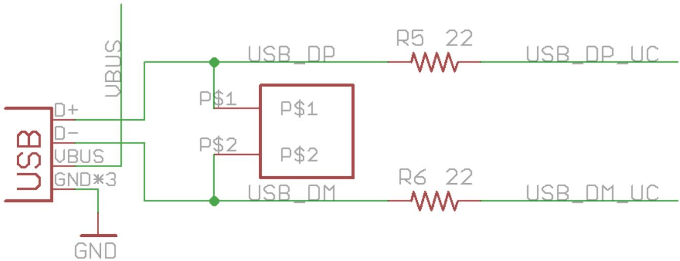
The USB data lines are terminated with 22 Ohm resistors. These data pins are also exposed via small through holes next to the USB connector and are labeled D+ and D-. The VBUS (+5VDC VCC of the USB port) is fed to the PMIC via a 3Amp Schottky diode ([SS3P3](#)). The VBUS pin is also available via the unpopulated header hole on the top-right side of the Electron.
