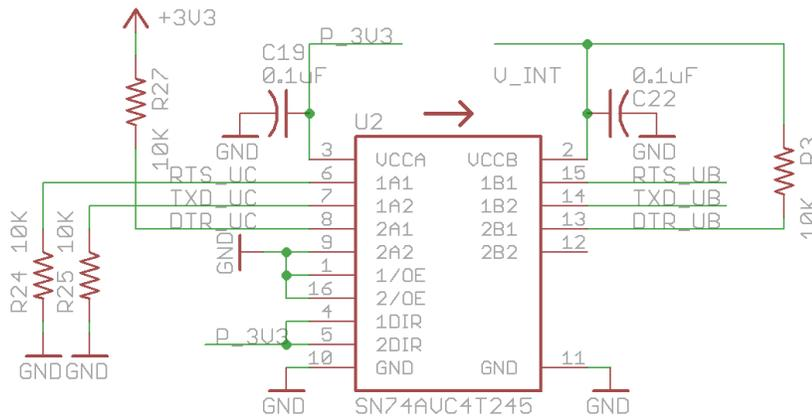
Since u-blox module's communication interface operates at 1.8VDC, while the STM32F205RGT6 microcontroller operates at 3.3VDC, we need voltage translators in-between them. This is achieved with two [SN74AUC4T245](#) non-inverting buffers. The default state of the USART pins is set with the help of pull-up and pull-down resistors, and the unused input pins are tied to GND.
