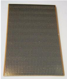
Experimental board in euro measurement, flash-gold plated (better for soldering "lead-free"). FR2 Phenolic paper
