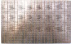
The strip raster is interrupted every 3rd hole. One-side copper layer, flash-gold plated (better for soldering "lead-free"). FR2 Phenolic paper
