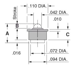
**Description:** Spring-Loaded Insulated Spring Pin Spring-Loaded Header Initial Height .100" (2,54mm) Single Row Surface Mount Plating Code: 22 Shell Plating: 20µ" Gold over 100µ" Nickel Inner Spring Plating: 10µ" Gold Packaging: Packaged in Bulk
