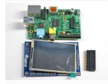
The easiest way to attach the header is if you have a Raspberry Pi as a 'stand' - make sure its powered off & unplugged!
