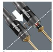
The Impaktor holder with ring magnet additionally holds longer and heavier screws absolutely securely. This enables a speedy and dependable positioning of the screw. It is also ideal for abovehead work. Should the magnet function not be required in a particular situation e.g. when working with metal, it can be extracted from the screwdriving area and can thereby be "disabled". Mainly used in manual power tool applications.
