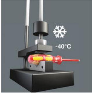
Impact strength tested at  $-40^{\circ}\text{C}$ , guaranteeing safety even under extreme conditions.
