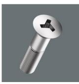
TRI-WING® The screwdriving system is mainly found in aviation and household technology (here e.g. on live components). The asymmetric arrangement of the three profile flanks prevents the use of anything other than the original tools. The high-precision Wera profile design ensures a secure fit of the tool in the head of the screw. The blades are manufactured out of bit material. The Wera know-how with regard to the hardening technology ensures a long service life of the tool.
