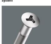
TRI-WING® The screwdriving system is mainly found in aviation and household technology (here e.g. on live components). The asymmetric arrangement of the three profile flanks prevents the use of anything other than the original tools. The high-precision Wera profile design ensures a secure fit of the tool in the head of the screw. The blades are manufactured out of bit material. The Wera know-how with regard to the hardening technology ensures a long service life of the tool.
