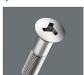
TRI-WING® The screwdriving system is mainly found in aviation and household technology (here e.g. on live components). The asymmetric arrangement of the three profile flanks prevents the use of anything other than the original tools. The high-precision Wera profile design ensures a secure fit of the tool in the head of the screw. The blades are manufactured out of bit material. The Wera know-how with regard to the hardening technology ensures a long service life of the tool.
