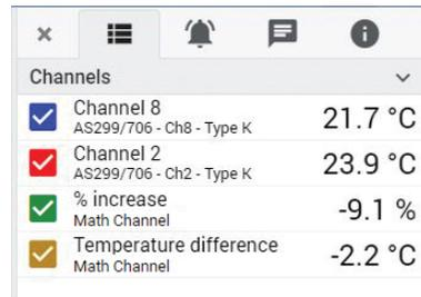
A screenshot of the 'Channels' panel in PicoLog 6. It shows a list of four channels with their respective values and units. Each channel has a checkbox on the left, which is checked for all of them.
