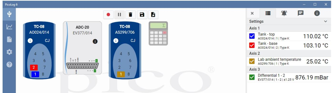
A screenshot of the PicoLog 6 main interface. The central area shows three device icons: two TC-08 (AO024/014) and one ADC-20 (EV377/014). The right-hand panel shows the 'Settings' view with three axes of data being logged. The top axis shows 'Tank - top' at 110.02 °C and 'Tank - base' at 103.10 °C. The middle axis shows 'Lab ambient temperature' at 25.02 °C. The bottom axis shows 'Differential 1 - 2' at 876.19 mBar.
