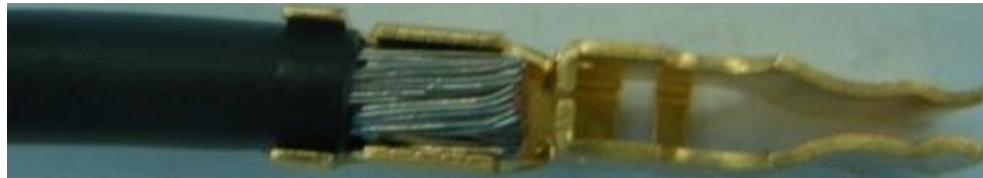
Picture 4. Wire and Terminal before Crimping
