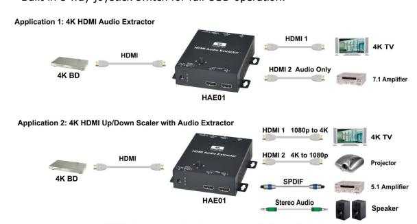
HDCP 2.2 to 1.4 and 4:4:4 to 4:2:0 and Up/Down Scale Capable Full OSD operation for all setup/EDID management
