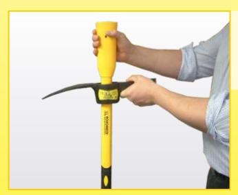
Insert the thinner end of the handle through the large end of the hole of the head
