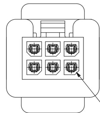
OVERMOLDER MAY UTILIZE AT THEIR DISCRETION A CAP SIMILAR TO THIS DESIGN TO PREVENT OVERMOLDING MATERIAL FROM ENTERING WIRE CRIMP AREA OF HOUSING
