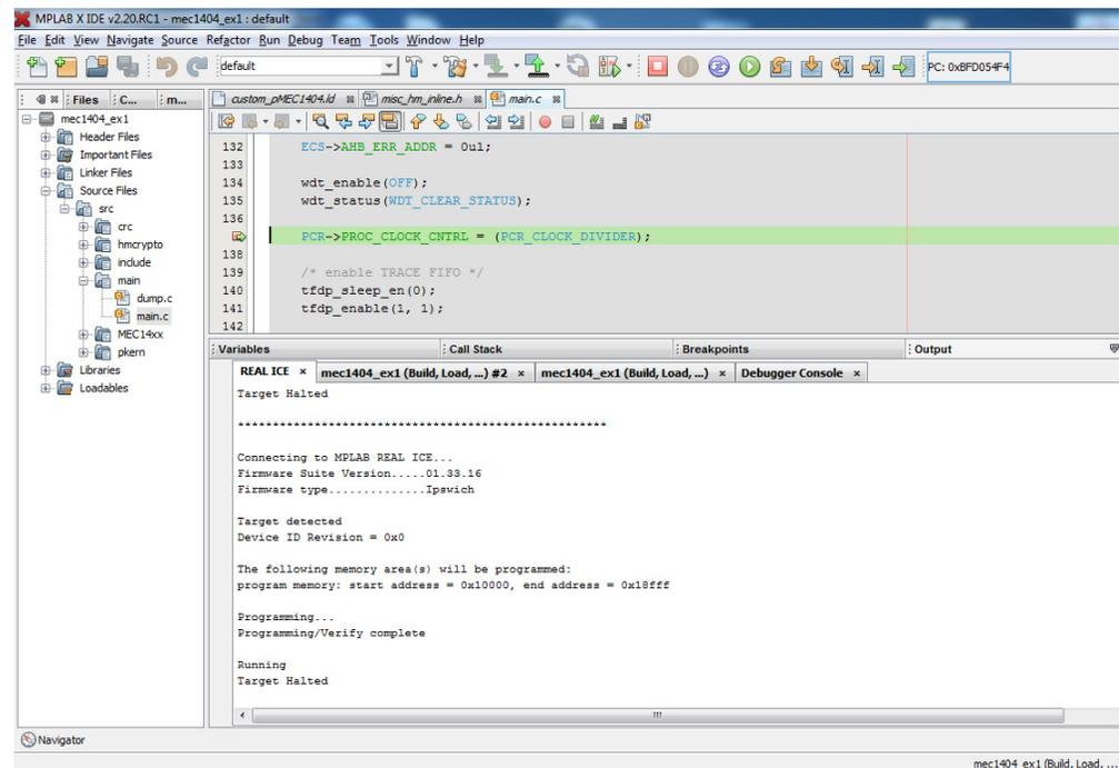
User can debug code via “step over”, “step into” or “continue”.
