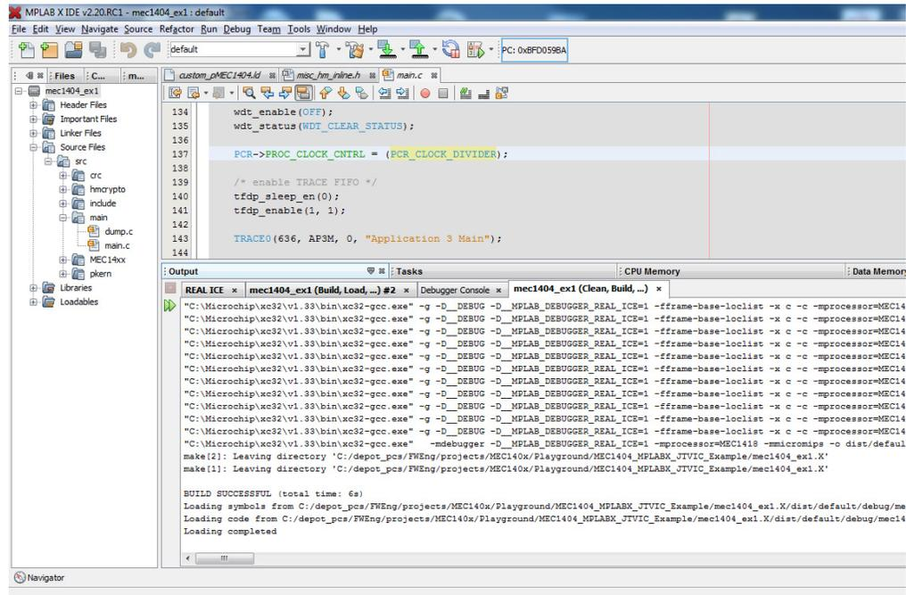
A successful build, if Real Ice is connected, will establish the connection and download the code to the target board for debugging.
