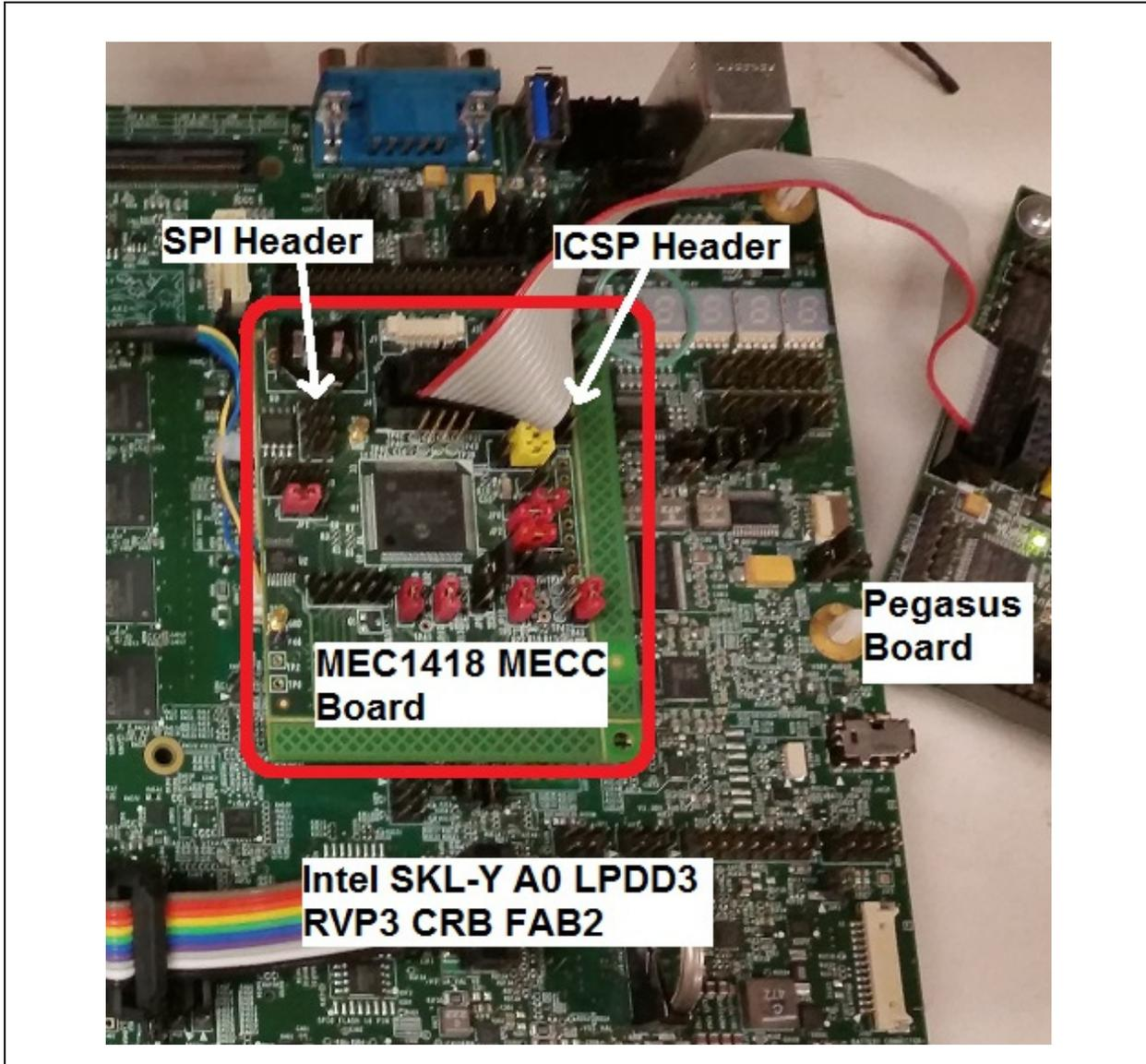
1. Connect Microchip Real ICE to the MECC J1 with RJ-11 to ICSP adapter
