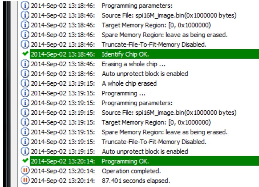
11. The firmware is now stored in the external SPI flash device. Please remove the JP9, and do a power cycle (please make sure to wait long enough to have power supply discharge before re-powering the MECC board). The new firmware should be loaded by the MEC141x internal ROM to the internal SRAM and start executing.
