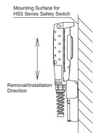
Make sure that the HE9Z-GP15 actuator is inserted completely into the safety switch. Avoid any foreign objects between the actuator and safety switch as they may interfere with the plastic spring, resulting in possible damage to the actuator.
