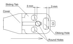
When using a hasp such as shown below, make sure that the hasp is installed in round holes not in the oblong hole. Otherwise the sliding tab may slide 3 mm or more. Check periodically that the narrow gap between the jaws is not widened, so that the HS9Z-PH5 does not fall off from the hasp.
