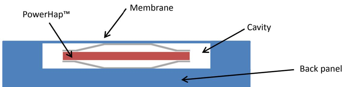
In this case the PowerHap actuator is clamped between a thin, flexible membrane and a rigid back panel. By applying a voltage, the actuator elongates and consequently deforms the membrane.
