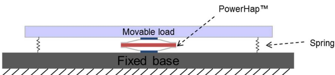
By applying a voltage to the actuator, it elongates and therefore moves the load. This movement can be felt by the user. For a maximal haptic feedback, the rear panel needs to be as heavy as possible. Otherwise the PowerHap actuator will not only move the load but also the rear panel and therefore a part of the performance is lost.
