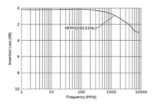
Common Mode Insertion Loss Characteristic (Typical Value)
