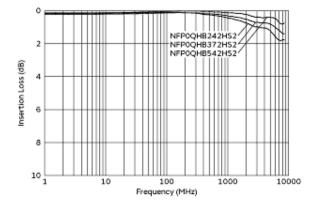
Common Mode Insertion Loss Characteristic (Typical Value)
