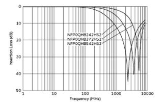
Common Mode Insertion Loss Characteristic (Main Items)(Typical Value)
