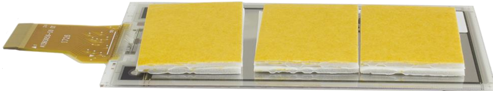
Figure 4 – ePaper Display, Two Layers of Double-Sided Tape on Bottom Side
