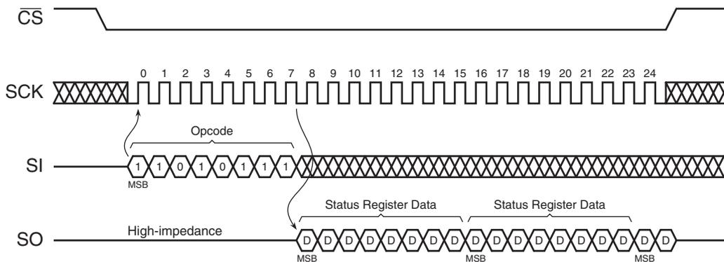
**Figure 25-10. Manufacturer and Device Read (Opcode 9Fh)**
