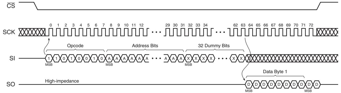
**Figure 25-5. Buffer Read (Opcode D4h)**
