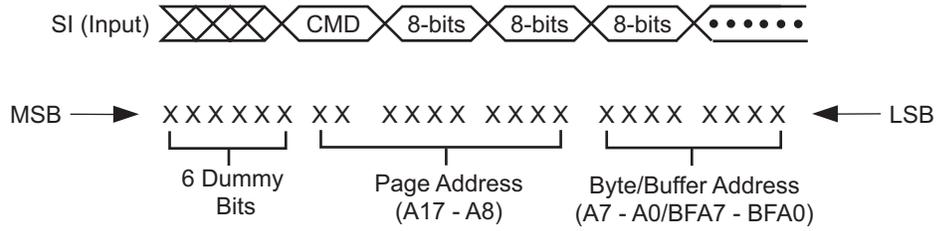
**Figure 21-3. Command Sequence for Read/Write Operations for Page Size 264 bytes**
