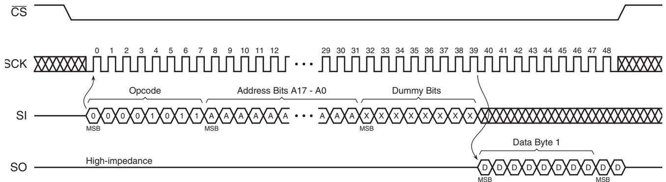
Figure 25-3. Continuous Array Read (Opcode 01h or 03h)
