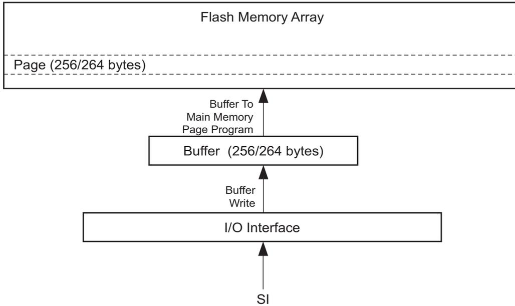
Figure 23-2. Buffer Write
