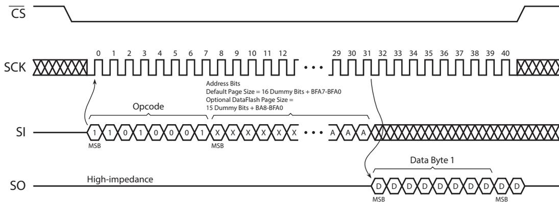
**Figure 25-7. Read Sector Protection Register (Opcode 32h)**
