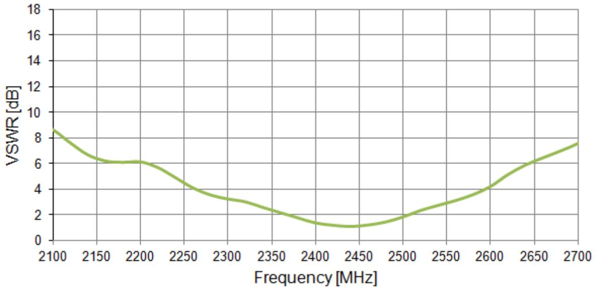
**Figure 4.** VSWR of the FXP840 antenna from 2100 MHz to 2700 MHz.
