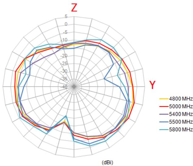
**Figure 14.** 2D Radiation Pattern at 5800MHz band
