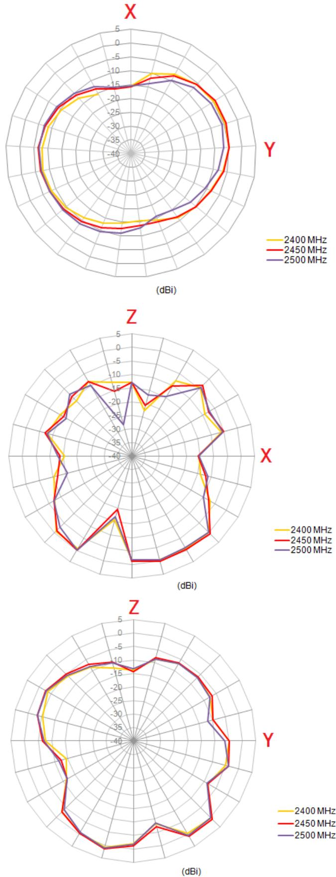
**Figure 13.** 2D Radiation Pattern at 2400MHz band
