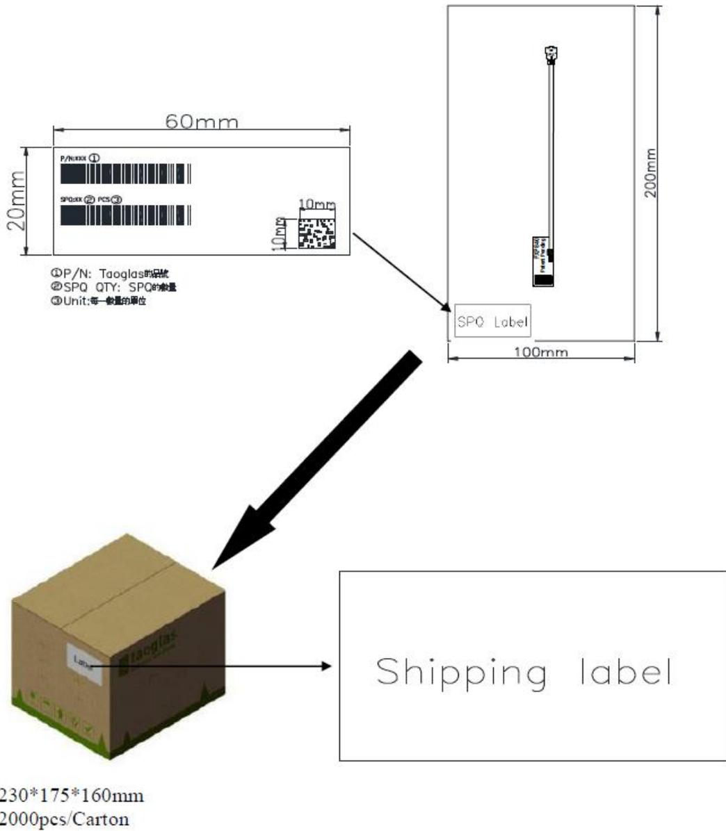
**Figure 16.** Package of the FXP840 Antenna.
