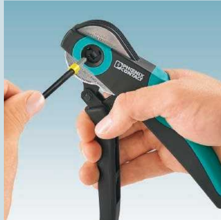
The CRIMPFOX CENTRUS crimps insulated, non-insulated and twin ferrules in a cross-section range of 0.14–6 mm 2 or 0.14–10 mm 2 .
