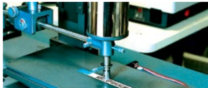
Abrasion resistant: after a 1kg sanding device was passed over the laminated labels 50 times, the text was unaffected.
