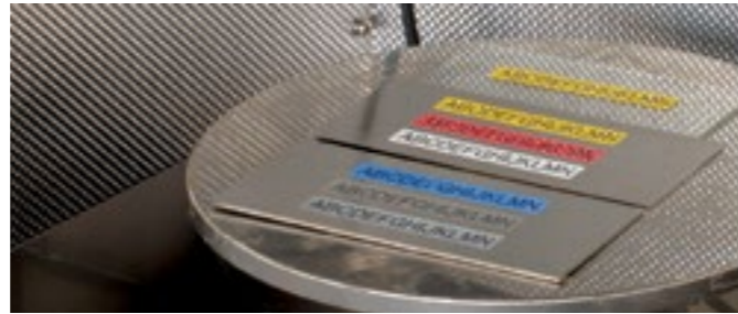
Fade resistant: after laminated labels were placed in a fade-inducing chamber to simulate a year in sunny surroundings, the text was unaffected.
