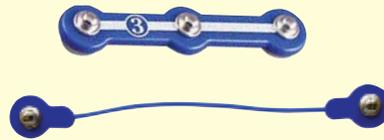
The blue **3-snap wires** and **jumper wires** (blue & orange) are wires used to connect components. They are used to transport electricity and do not affect circuit performance. The 3-snap wires make rigid connections, while the jumper wires make flexible connections.
