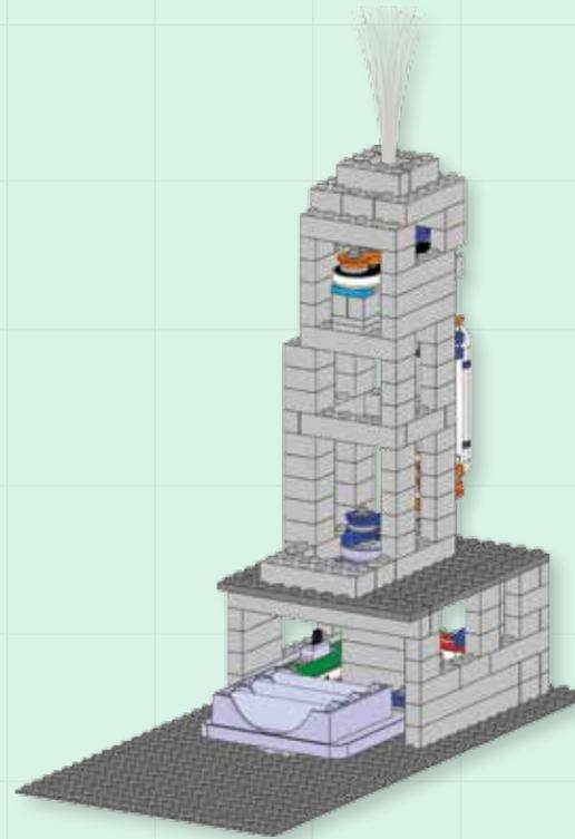
Build the circuit as shown, and turn on the slide switch (S1). The four LEDs (D8, D9, D11, & D12) and lamp (L4) light, and the melody IC (U32) plays tunes. The 3D snaps allow the blue and blink red LEDs to be rotated to shine in different directions. Dim the room lights for best effects. You can omit the sound by removing the melody IC (move the blink red LED (D11) to where the melody IC was).
