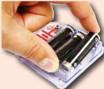
When installing a battery, be sure the spring is compressed straight back, and not bent up, down, or to one side.
