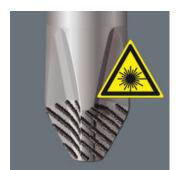
A precisely-focused laser creates a sharp-edged surface structure. This laser treatment results in an edge hardness of up to 1000 HV 0.3. Wera Lasertip "bites" itself into the screw head and prevents any slips out of the recess. It is available for screwdrivers for Phillips and Pozidriv slotted, screws.
