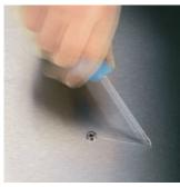
It happens time and time again that the tip slips out of the screw head when screwdriving, sometimes damaging valuable surfaces or even causing injury. The tips of the Wera Lasertip screwdrivers are microscopically roughened by means of a laser. This rough surface literally "bites" itself firmly into the screw head. Slipping out becomes a thing of the past.
