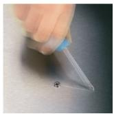
It happens time and time again that the tip slips out of the screw when screwdriving, head sometimes damaging valuable surfaces or even causing injury. The tips of the Wera Lasertip screwdrivers are microscopically roughened by means of a laser. This rough surface literally "bites" itself firmly into the screw head. Slipping out becomes a thing of the past.
