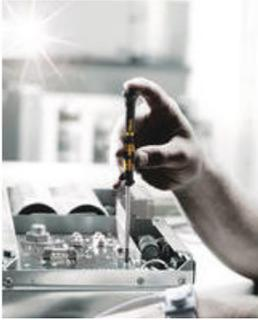
When doing screwdriving jobs on electronic components (like e.g. smartphones and tablet PCs), there should be no electrostatic discharge as this could cause malfunctions and a complete failure. Therefore, tools that are secure against electrostatic discharge are indispensable.
