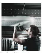
With the Joker, you can now loosen and tighten nuts and bolts, in situations where conventional tools fail. Particularly in confined spaces, where conventional open-jawed wrenches cannot be used. The combination of limit stop and small return angle enables eff ective work, even on screw pipe connections.
