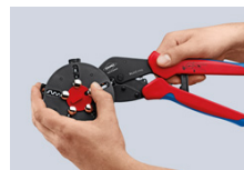
Changing the crimping dies: unlock the magazine position, take out the set of dies which the pliers have been pushed on
